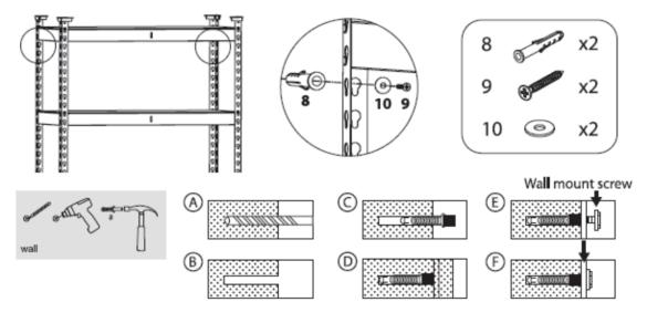
NOTE: Supplied wall plugs are only suitable for use in masonry walls. CAUTION: When drilling into walls, always check for hidden wires or pipes, etc.
