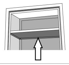
Screw the top panel to the inside of the cabinet as indicated by the arrows.
