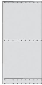
1 x Rear Wall (install this way up & face detail towards inside of cabinet)
